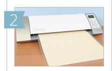
Position a piece of paper or cardstock onto a cutting mat and load it into your Silhouette electronic cutting tool.
