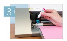
Select a Silhouette sketch pen, remove the cap, and place the pen into the blade holder of your Silhouette electronic cutting tool.
