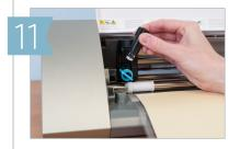
Load the blade into the blade holder of your Silhouette electronic cutting tool. Click "Cut" in the Silhouette Studio® cut settings menu.
