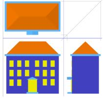
A standard orthographic drawing normally comprises three views: front, top, and side.
