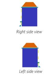
An orthographic projection includes the front and plan views of an object and will include either or both the left and right hand sides as well. A projection would be complete when it includes the rear and bottom views too, making a total of six 2D views to illustrate the 3D object.
